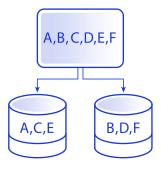
▼ RAID 1 – A basic form of mirroring providing excellent redundancy at the cost of space. In a two-drive system, a complete copy of the data on one drive is written to the other. This redundancy is enhanced with each drive added. Since all data must be mirrored across all drives, total space on the system will be limited to just the space of the smallest drive in the system.
